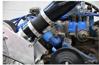
The plumbing is designed to work with a swivel thermostat housing. Such as this one from Scott drake. Part number B-F434 for 64-73 390-428cu.
