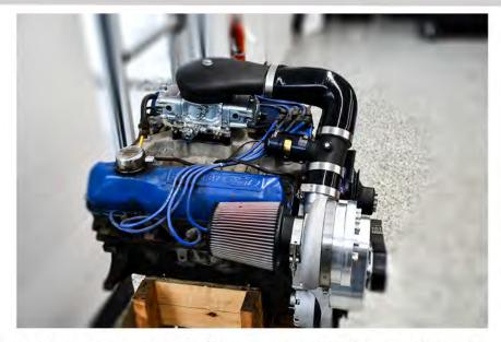
Install carb hat and charge tube. The couplers are purposely long to accommodate a variety of configurations, so trimming may be required. Loosen the v-band clamp to rotate the compressor housing. When finished. Do not overtighten. 1/8-1/4" of thread showing. Just so the housing is
